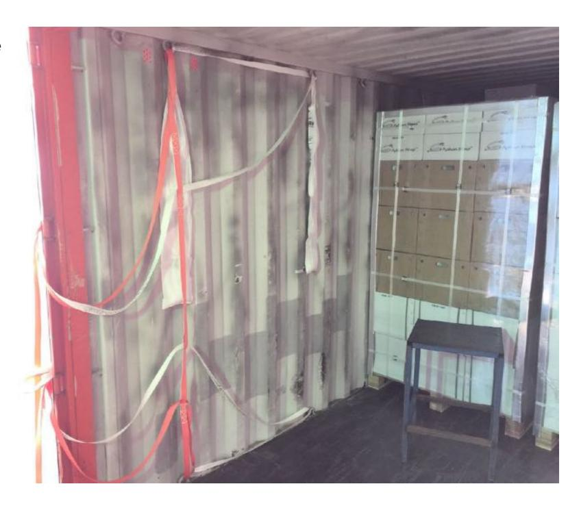
After your container is fully loaded, bring the four pairs of belts together and apply the 4 buckle.
