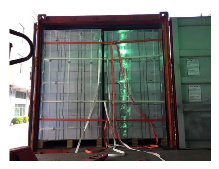
Use the S-50 tensioner to pull the belts real tight to secure the cargo.
